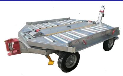
The ACD1600-3 eliminates the need for manual setup of ULD locks. The locks automatically retract when a ULD rolls over it and returns to the locked position once the ULD has cleared.
